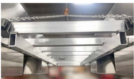
Featuring a uniquely strong understructure supported by standard longills and cross members
